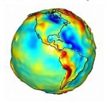
country there was a campaign to observe GPS on NAVD 88 benchmarks. GPS on benchmarks (GPSBM's) were used as control to make Geoid99, Geoid 03 and Geoid 06a, Geoid 09, Geoid 2012B, Geoid 2018.
