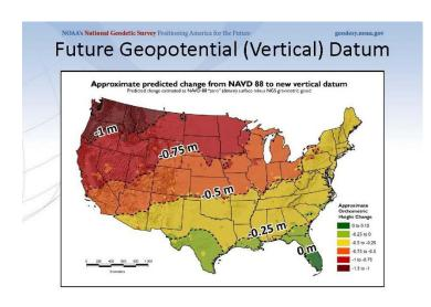
The latter will be primarily accessed via GNSS and the geoid. There will be an accurate continental gravimetric geoid which aligns with the Terrestrial Reference Frame of 2022 (TRF2022) and global mean sea level (GMSL). The varying nature of gravity over time will be monitored via the Geoid Monitoring Service (GeMS).
